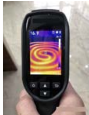
Check Floor Heating
